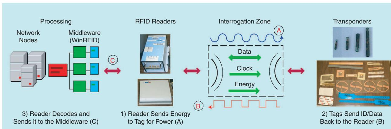
**[FIG1]** An RFID system. (Figure courtesy of UCLA-WINMEC.)
