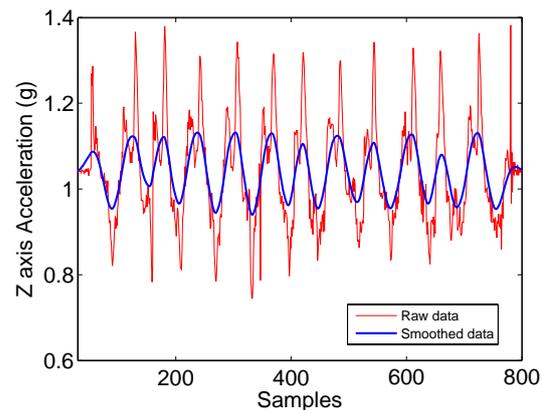
Figure 2. Accelerometer output from a gym machine (Sampled at 40Hz)
