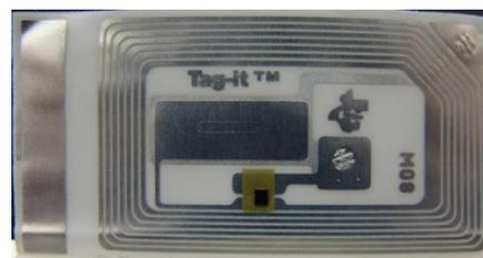
Figure 5: Zebra RFID Tag Circuit
