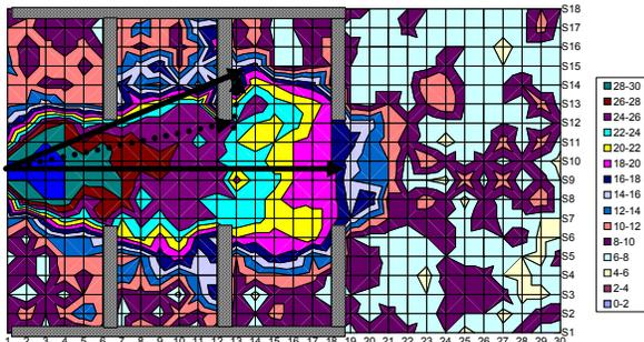
Fig. 14. Readout signal distribution of the SAW reader at the center devices was observed around the office.
