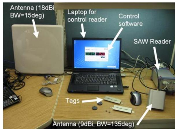
Fig. 5. Reader, Tags, Antennas and Operating software
