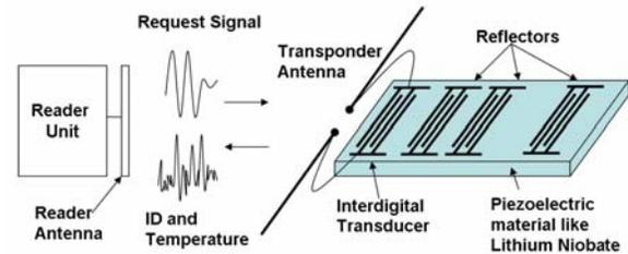
Fig. 4. Principle of SAW technology
