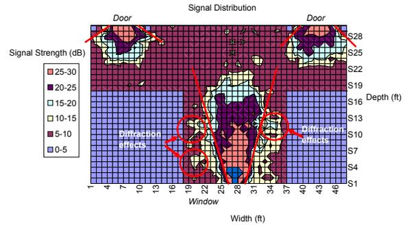
Fig. 13. Readout signal distribution of the office. Good signal is 25dB or over.
