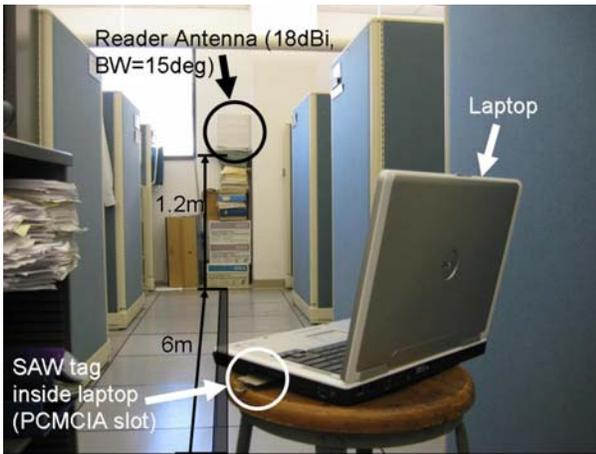
Fig. 9. Detecting ID and temperature
