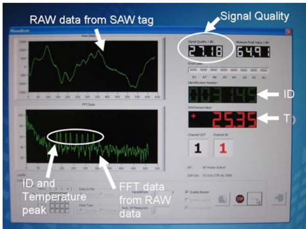
Fig. 6. Detecting ID and temperature
