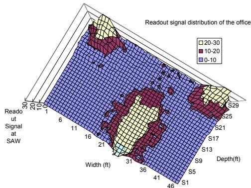
Fig. 12. Readout signal distribution of the office. ID and Temperature; >20, ID only; >10
