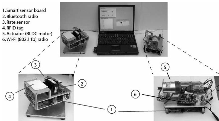
Figure 3. Smart sensor platform test setup
