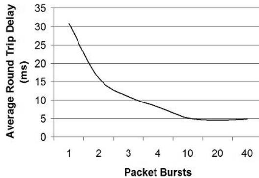
Figure 5. Average round trip delay with varying packet bursts for WiFi
