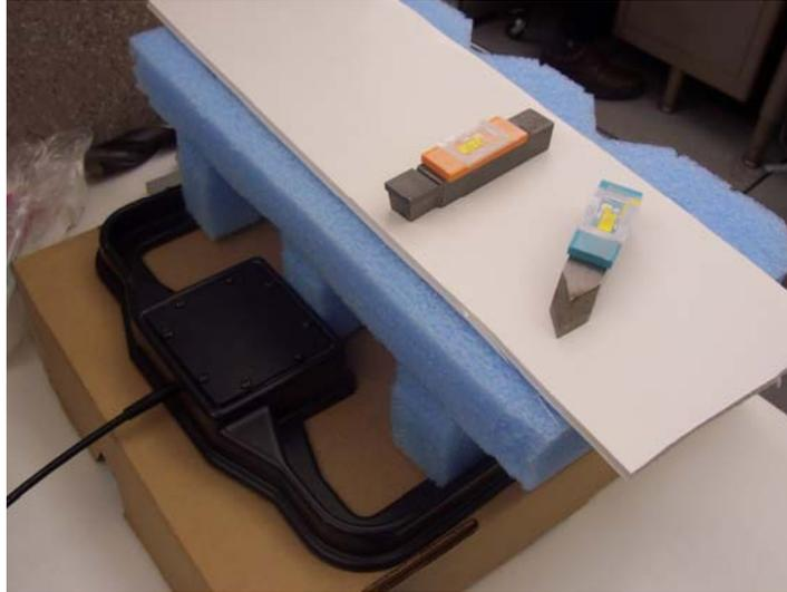
*Figure 4: Tags attached to tools and antenna*
