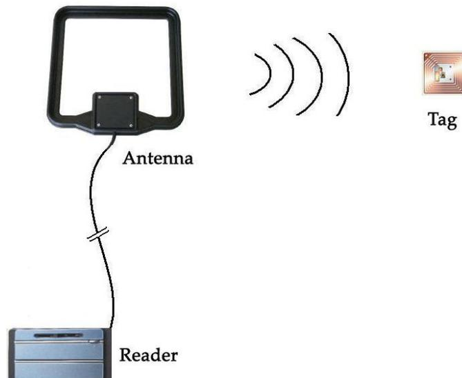
*Figure 1: Typical RFID System*
