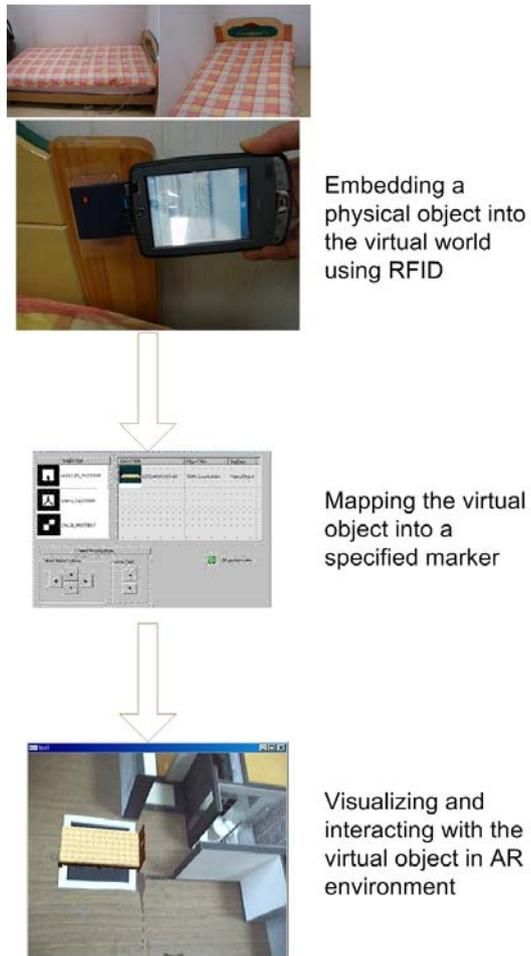
Fig. 2. A scenario: integration of AR with RFID for hyperlinking physical object with virtual ones in the cyber home modeling
