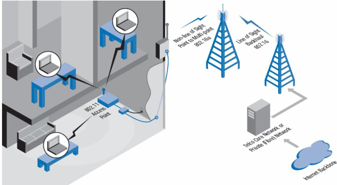
Figure 1: 802.16 for broadband wireless access (Source: Intel)
