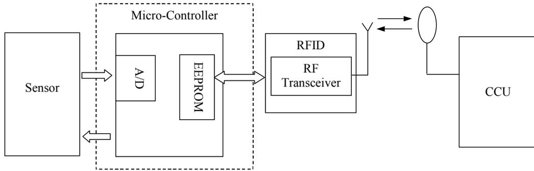
Fig. 1 Architecture of Intelligent Wireless Sensor System
