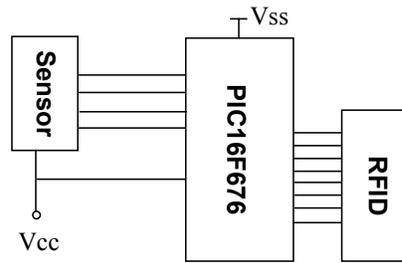
Fig. 3 Schematic of Micro-Controller
